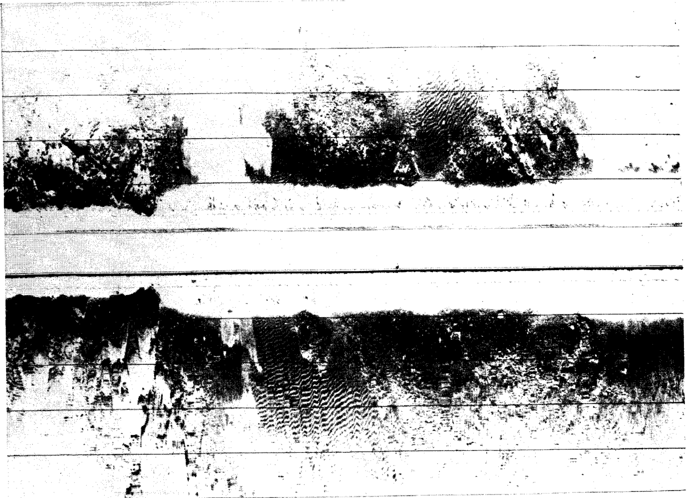
FIGURE 2. Dual-channel 200-kHz side-scan record made near Marblehead, Mass. Scale lines are spaced at 50-foot (15.5-meter) intervals. Ripple areas near the center are sand waves, dark areas to the left of the photo are sharp rock outcrops, smaller rock outcrops are seen on the right side. Blank areas represent smooth mud bottom with low acoustic backscatter.
