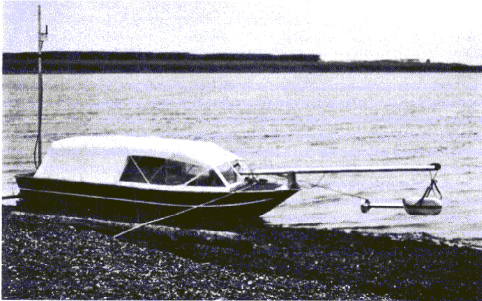
Fig. 11: Combined side scan sonar/sub-bottom profiler mounted off the bow of a small survey vessel. Photo courtesy Nortrek.
