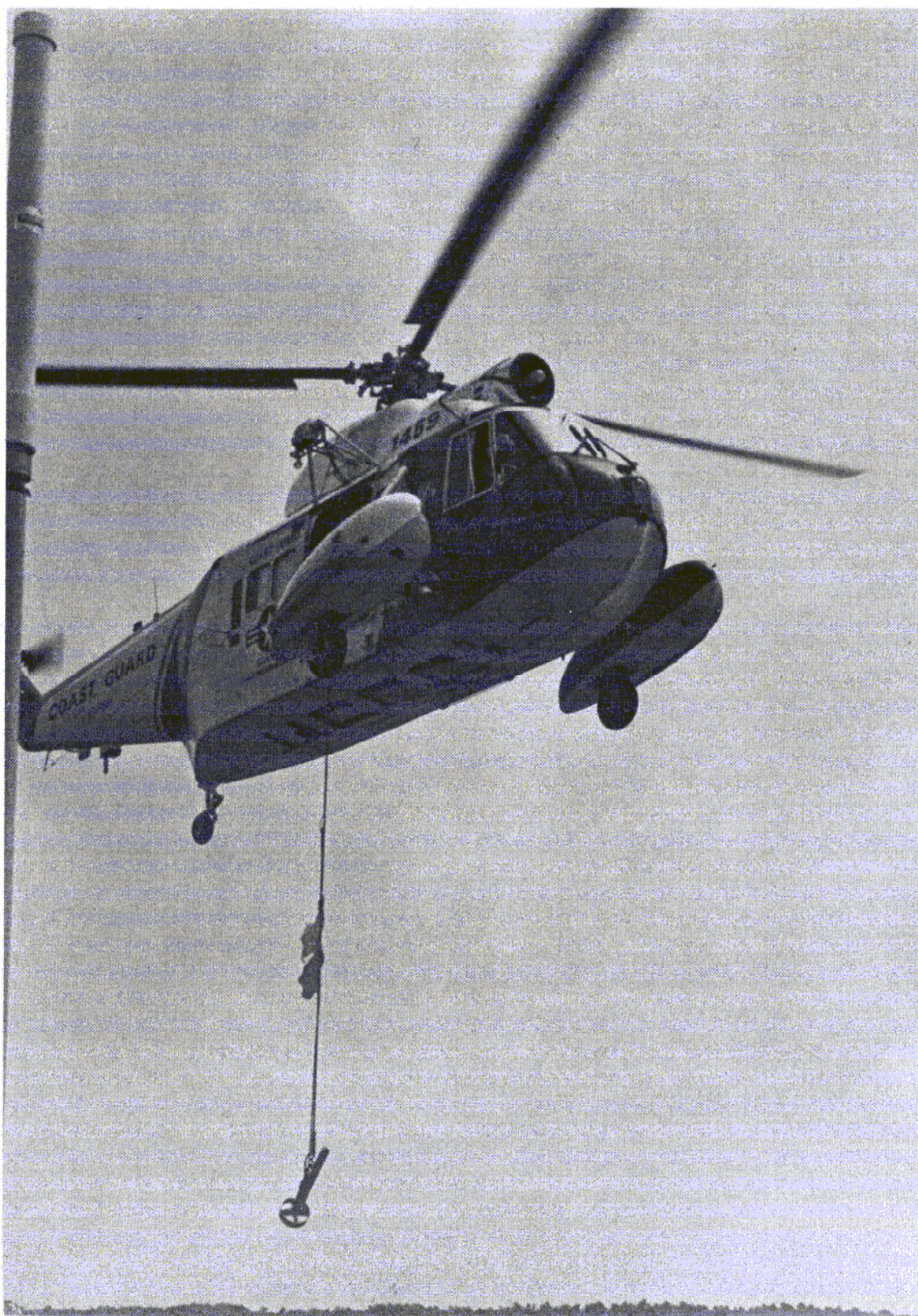
Fig. 14: Klein side scan sonar towfish shown in a successful sea trial with a helicopter. The towfish was towed with a special high strength lightweight cable.
